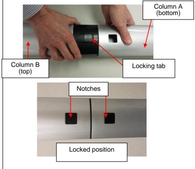
5. Place scale platform C on its side and place Column B on its side, perpendicular to the platform. The front of the display head on Column A should be facing forward and above scale platform C.
