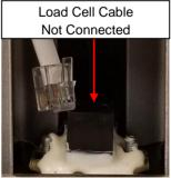
2. Inspect the load cell connector cable to ensure it is completely plugged into the RJ jack. If cable was plugged in, unplug and plug in again until it clicks into place. After checking connection, replace door at the back of the platform base.
