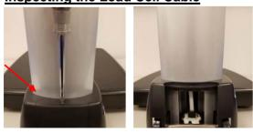
1. Using a Phillips screwdriver, remove the door at the back of the platform base.
