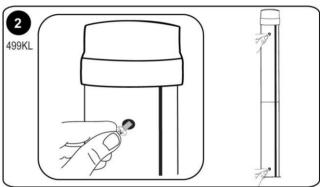
Position the large keyhole slots on the height rod over each screw head. When positioned correctly over both screws, gently slide the 499KLROD all the way down, in order to secure the keyhole locks.
