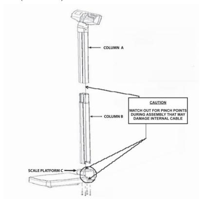
1. Carefully remove the scale platform and columns A and B from the carton. Place the scale platform and columns on a flat, level, and dry surface Remove the 4 column mounting screws and washers from the bottom of column B and set aside for assembly step 7.
