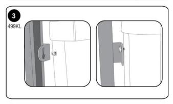
Tighten the screws with the enclosed wrench (wrench is provided with the 499KLROD).
