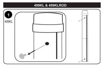
2. Insert the enclosed screws into the holes on the pillar.
