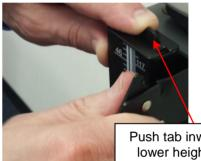
To lower height rod below 46 %", push the tab at the top of the height rod and gently lower the headpiece.
