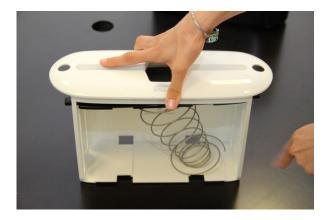
To fix the dislodged spring, simply push it back into the indented area at the bottom so it looks like this:
