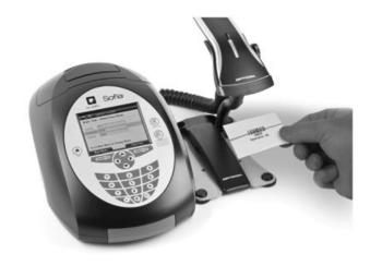
3. Input Patient ID or Order # using the barcode scanner or manually enter the data using the key pd.
