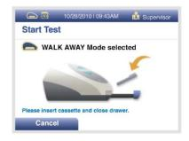
Verify that the correct mode, WALK AWAY or READ NOW, has been selected. Insert the Test Cassette into the drawer. Then gently close the door.
