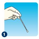
Remove the swab from its packaging, holding by the end of the applicator and identify the breaking point.
