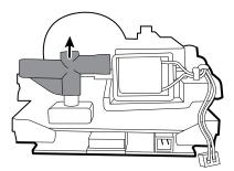
Lift the chassis assembly away from the circuit board assembly, and disconnect the battery contact harness from J2 on the main board.
