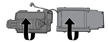
b. Lower the circuit board assembly into the front housing.
