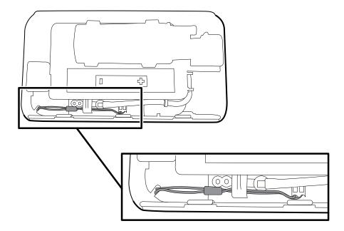
9. Align the inner chassis notches with the side panel guides, and align the dump valve manifold with the pressure transducer on the blood pressure board.
