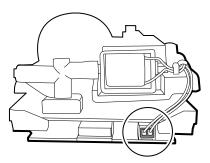
Disconnect the dump valve manifold from the pressure transducer on the blood pressure board.
