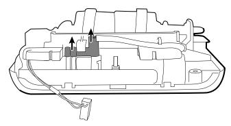
3. Disconnect the dump valve cable from J10 on the main board.
