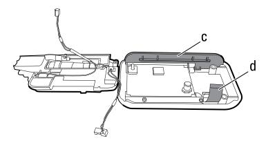
4. Insert the second side panel into the front housing, aligning the isolation bumpers with the PCBA mount pegs.
