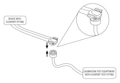
After a calibration test is complete, gently squeeze the side tabs of the port fitting and pull apart to disconnect the fittings.
